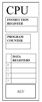
The Arithmetic Logic Unit (ALU) of a CPU can generally do basic arithmetic on binary numbers, and also logical operations such as checking equality -- whether two binary patterns are the same.
