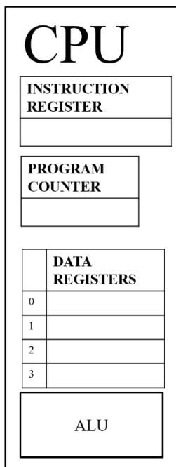
The Arithmetic Logic Unit (ALU) of a CPU can generally do basic arithmetic on binary numbers, and also logical operations such as checking equality -- whether two binary patterns are the same.
