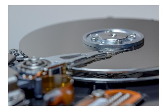
The magnetic read-write head, a magnet that reads and writes the state of the magnetic particles on the hard drive, must go very, very close to the surface to read the tiny particles. But if it actually touches the surface, it will do permanent damage. So the hard drive must be carefully designed to limit the movement of the heads and platters as much as possible – the less movement, the less chance of damage.
