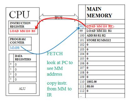
So, during Fetch, the address from the PC is sent to MM, which sends back whatever instruction is at that address. This instruction is copied into the IR.
