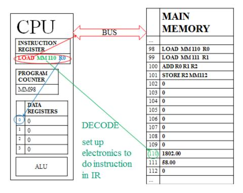
For example, if the instruction says to have the ALU add numbers, then the data registers containing those numbers must be activated, as must the adding component of the ALU, and it must be set to put its result into the correct data register. If the instruction says to copy data from MM to a Data Register, the address of the data must be sent over the bus, and the bus set to copy the data into the correct register when the MM sends it back.
